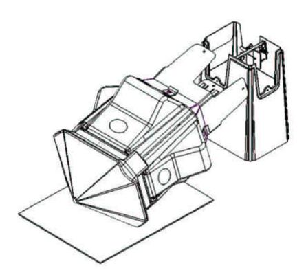
*All models* Remove the Base Shield from the Terminal Bracket. It is held in place with a wing nut. The wiring diagrams for Installation are on this part.
