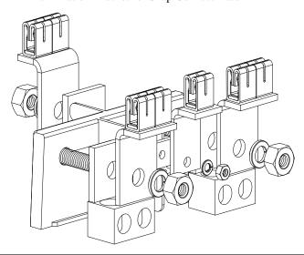
Set the Base in place with all utilities running through the bottom Plate and attached to it as appropriate. Tighten the 4 hold down bolts to secure the Base in place. These should be as tight as the mounting pad material and bolt system will allow. The PowerPort materials and method of construction will support as much hold down force as your bolt system can provide.
